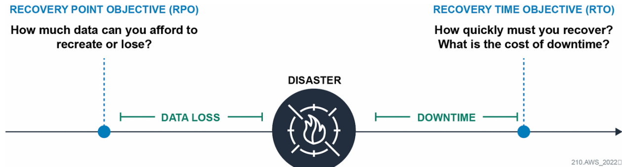
Figure 10: RPO and RTO. RPO relates to data loss in the event of a disaster; RTO relates to the amount of time systems are down.
