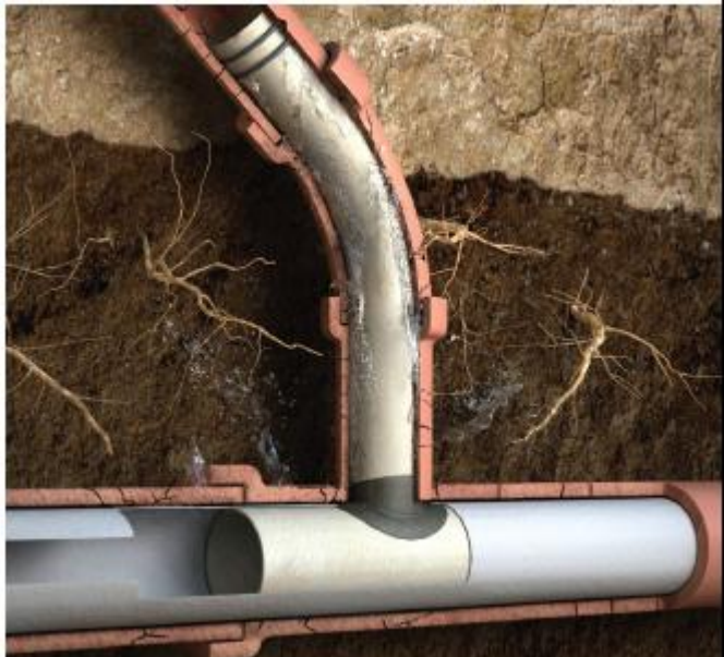
Watertight seal for lateral
