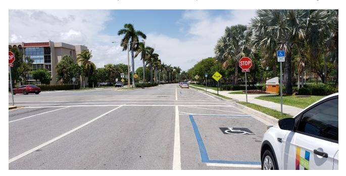
An angled parking configuration could also be an option, which may provide up to 72 parking spaces for this location. However, there would be a reduction of lane width, which will reduce the width of the current four lane road (two lanes in each direction) down to two lanes (one lane in each direction).
