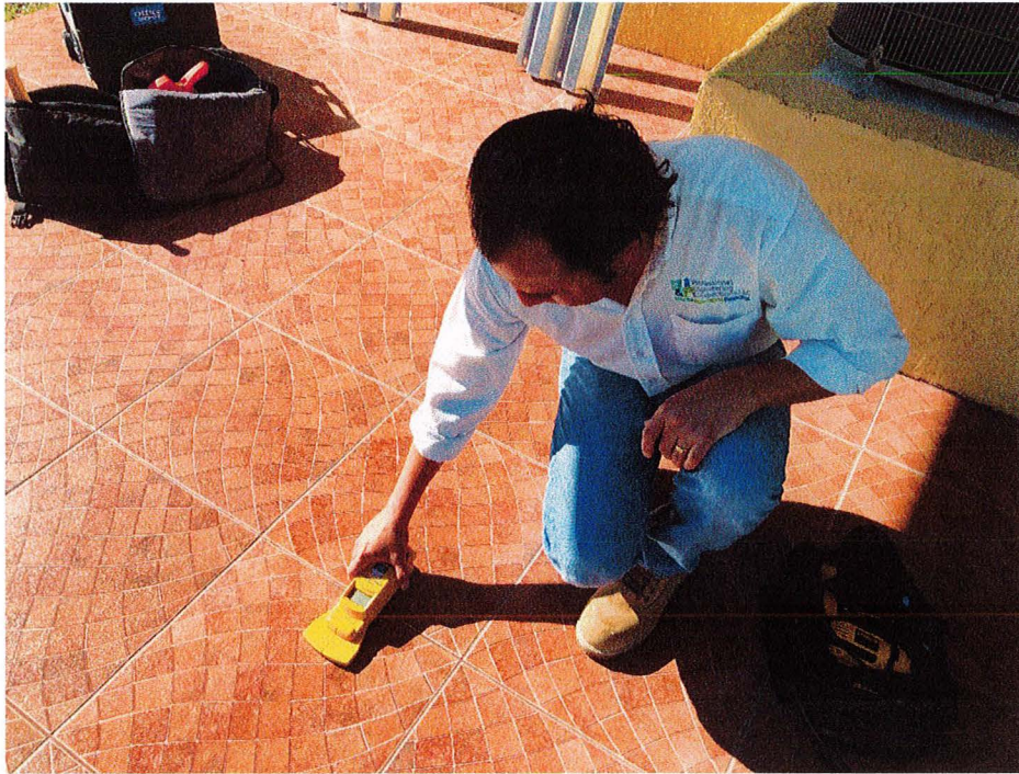
Photograph 11. Metal Scanning for rebar location
