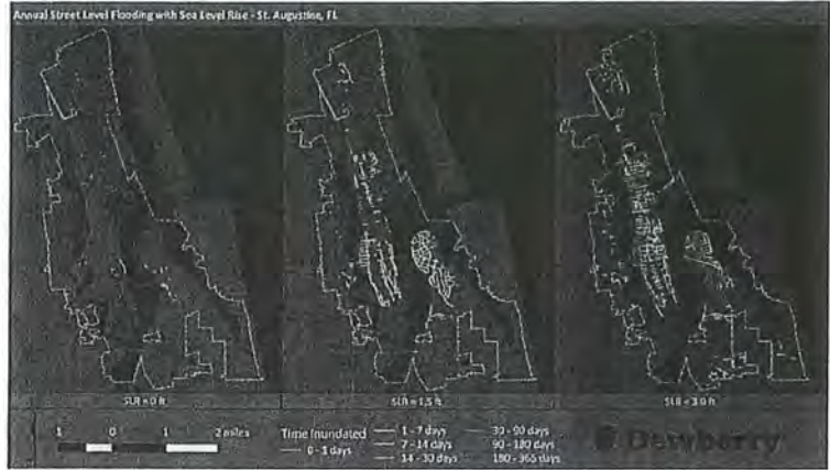
FIGURE 5. EXAMPLE CHANGES IN NUISANCE FLOOD FREQUENCY TO ROAD SEGMENTS PREPARED FOR ST. AUGUSTINE, FL.
